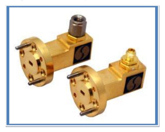
**Model SWC-101F-R1 and SWC-101M-R1** are W band waveguide to 1 mm coaxial adapters. These adapters offer convenient mean for waveguide to coaxial line connection for full W band operations. Both WR-10 waveguide to 1mm (F) and WR-10 waveguide to1 mm (M) coax adapters have less than 1.0 dB insertion loss and better than 15 dB return loss from 75 to 110 GHz. The waveguide to coax adapter family is offered to cover the frequency range from 18 to 110 GHz.
